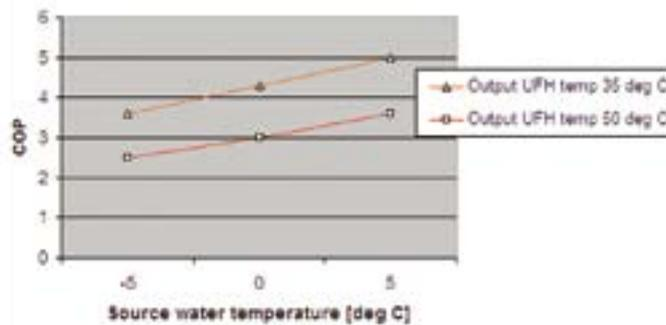
Fig. 3 – Coefficient of Performance (COP) graph for typical GSHP's
