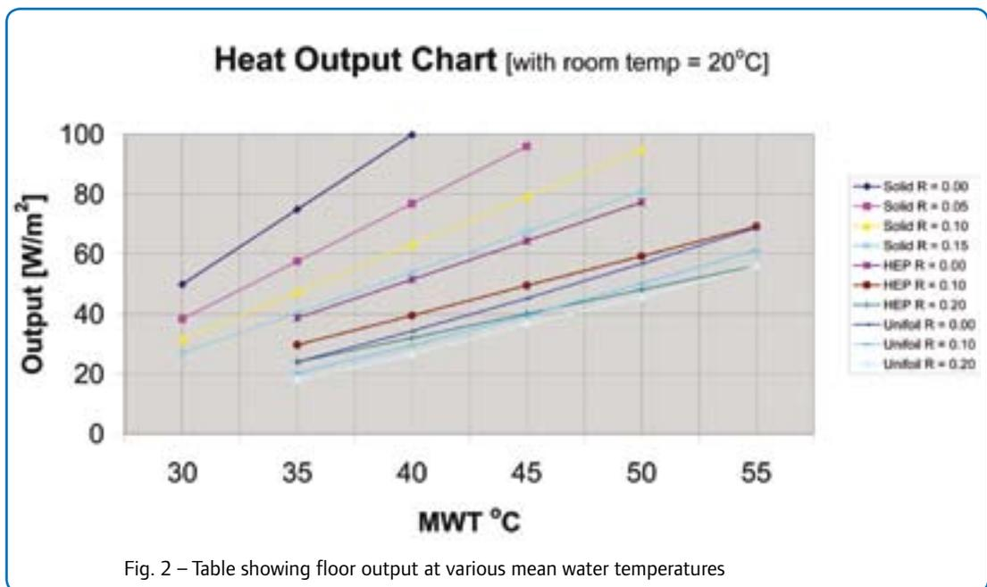
Fig. 2 – Table showing floor output at various mean water temperatures
