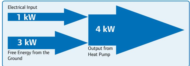
Fig 1 : Typical Energy Balance Diagram for GSHP
