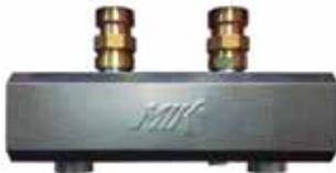
Depending on the system load, two sizes are available (up to 70kW and up to 165kW @  $\Delta t$  20 °C flow and return set up temperature). The heating appliances are then connected to the switcher, which provides an open circuit for the appliance system water to feed the heating distribution header. This can be supplied with 2 to 6 Grant zone pump kits for each heating and hot water circuit, as required.
